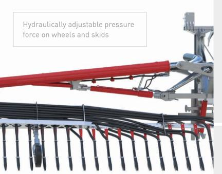
Flexible management of boom part width sections to implement different working widths with one linkage, without any overhang of the frame
